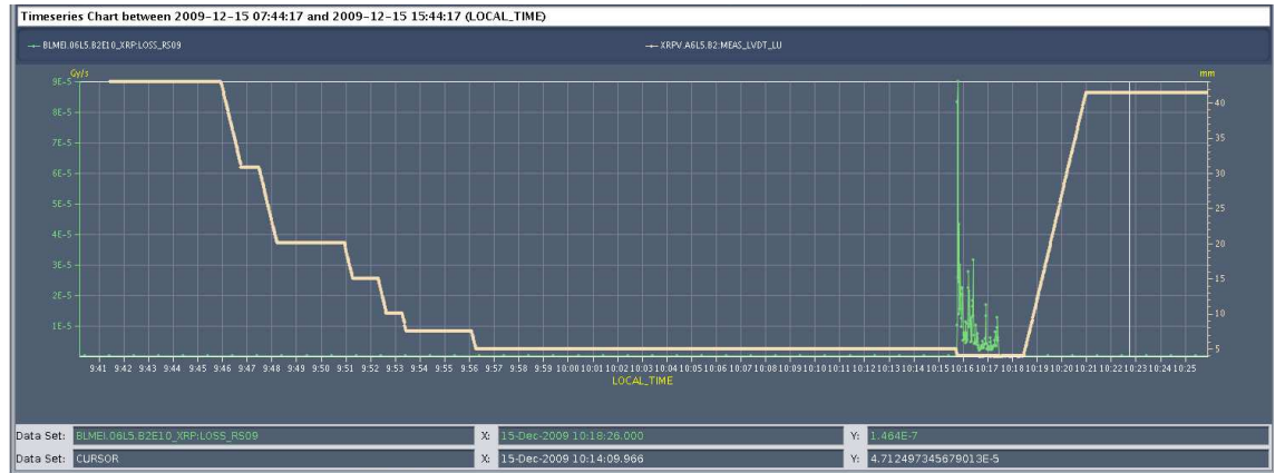
Figure 4: Overview of the scraping test on 15 December with beam 2. Orange curve: time evolution of the jaw position of RP-45-220-N-T (XRPV.A6L5.B2) at 215 m; green curve: time evolution of the BLM signal at 221 m (BLMEI.06L5.B2E10-XRP). At about 10:17:30 h the beam was lost.
