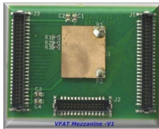
Figure 3 Trigger VFAT mezzanine
